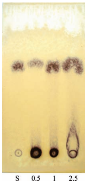
Figure 4. Thin layer chromatography analysis of the products of inulin hydrolysis by A. terreus purified inulinase. Standard (S), \alpha -fructose; reaction time, 0.5, 1, and 2.5 h.
